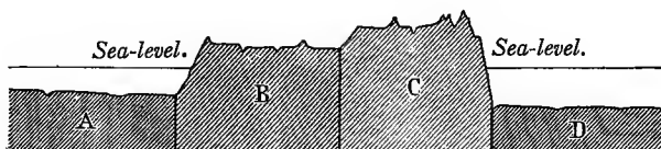
FIG. 2. Diagram illustrating the relationships between the denser suboceanic crustal blocks A and D and the light or terrestrial crustal blocks B, C, when in static equilibrium. (After Penck.)
